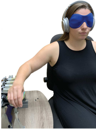
Fig. 4. The setup for the human subjects studies. Participants wore noise canceling headphones placed their right volar or dorsal forearm into the device. In the open response study and contact spacing study, subjects only placed their right volar forearm into the device and were also required to wear a blindfold.
